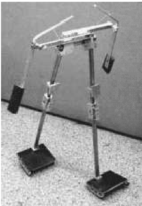
Figure 1.11: Photo of 3D passive dynamic walking robot of Collins.
