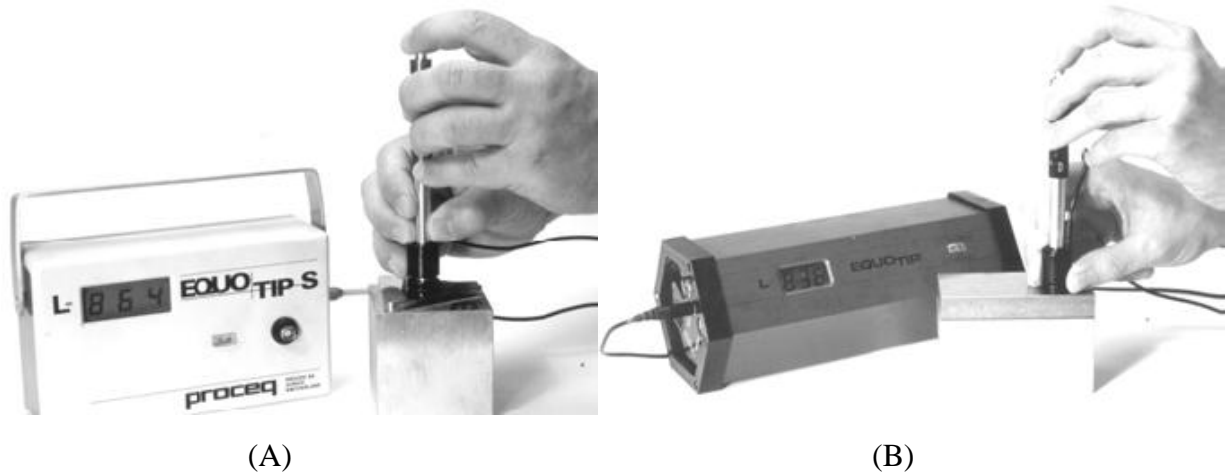
Figure 1.5 (A) First two models of EQUOTIP hardness testers. 1975 series, and (B) series of red hexagonal EQUOTIP, produced between 1978 and 1990 [1-7]
