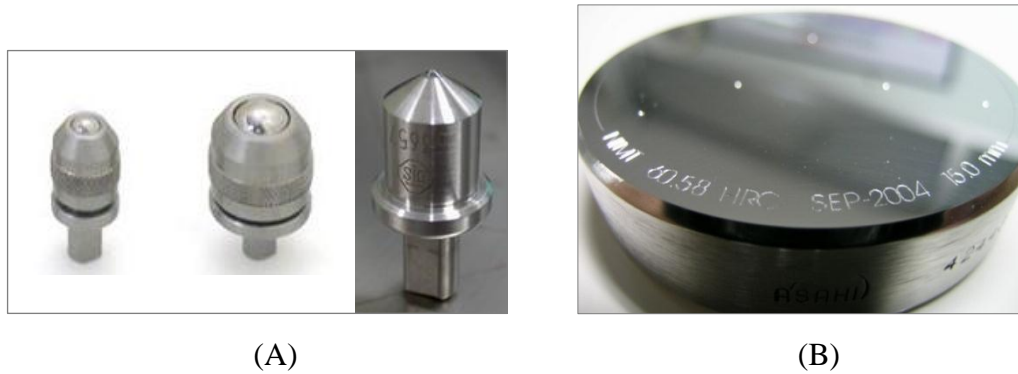
Figure 1.8 (A) The Rockwell indenters. (B) The certified hardness block
