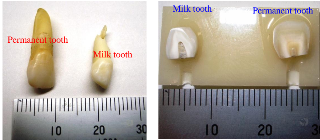
Figure 3.32 Two incisors teeth samples (milk teeth and permanent teeth) before cut (Left). The teeth were placed on substrate by epoxy glue (Right) with polished surface
