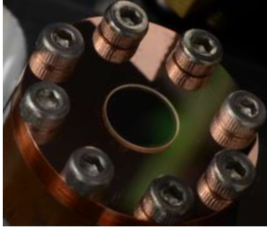
Fig. 5.4: Photograph of glued Yb:Lu 2 O 3 ceramic disk.
