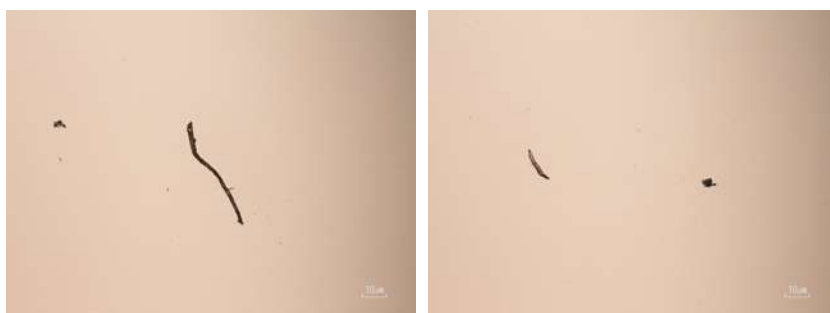
Fig. 4.33: Microscope images of a fresh 5 at.% Yb:LuAG ceramic plate.
