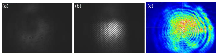
Fig. 6.2: Interference patterns of (a) and (b) soldered Yb:Lu 2 O 3 ceramic disk, and (c) glued Yb:Lu 2 O 3 ceramic disk.
