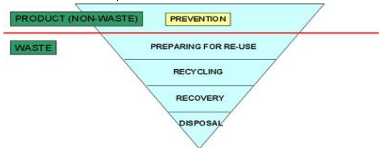
Figure 4. The waste management hierarchy according to the EU Waste Framework Directive, Source: European Commission, 2015
