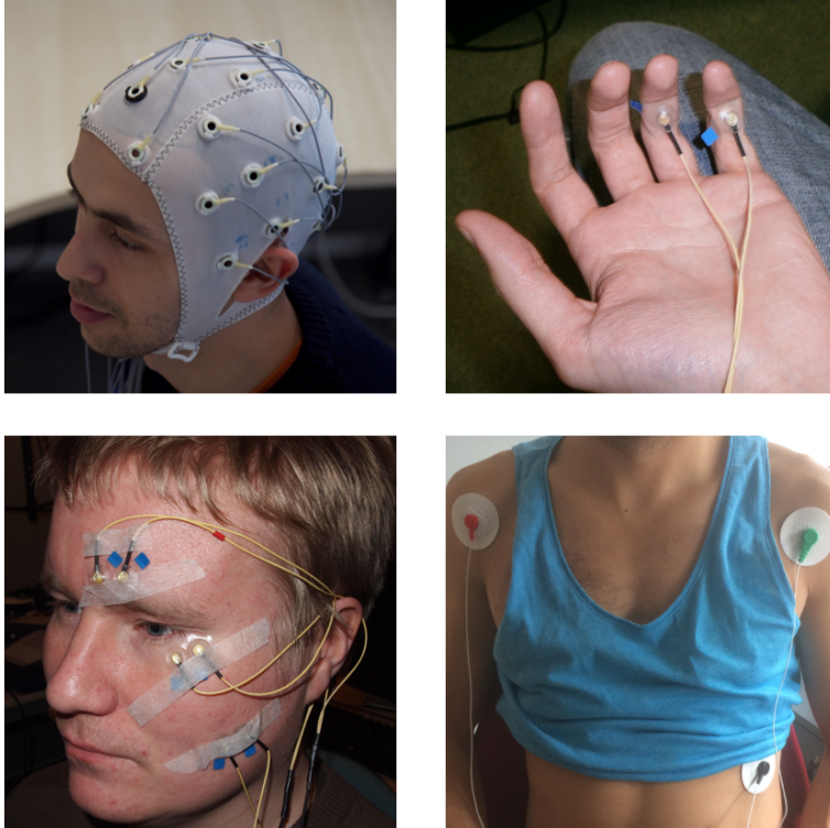
Figure 2.1: Physiological sensors used in this thesis. Electroencephalography (EEG, top-left), electrodermal activity (EDA, top-right), facial electromyography (fEMG, bottom-left), and electrocardiography (ECG, bottom-right).
