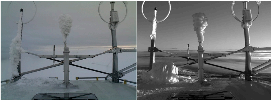
FIG. 8. Webcam images taken on (left) 7 and (right) 8 Jan 2013 from the top of the turbine nacelle, illustrating the visual assessment of icing and showing the ice load instrument with a cone of ice on it (middle of both images).
