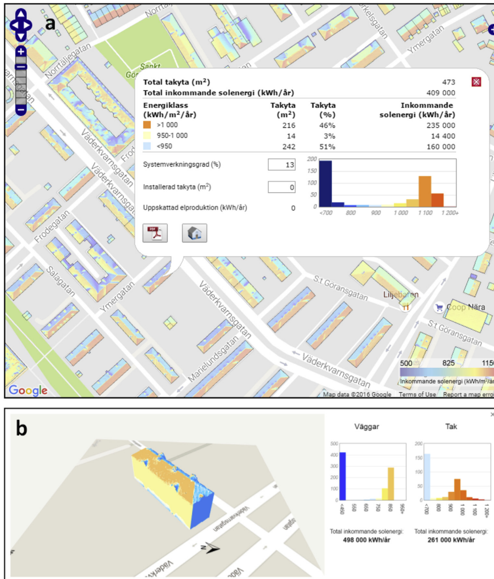
Fig. 11. SEBE results for an online application for rooftop irradiance in central Uppsala, Sweden, (a) pop-up window with statistics for one of the buildings, (b) 3D view of shortwave irradiance (walls and roof) for the building. ( www.uppsala.se/solkarta ) Meteorological data used in this example originate from a meso-scale model for solar radiation (STRÅNG, www.strang.smhi.se ) developed by the Swedish Meteorological and Hydrological Institute (SMHI).
