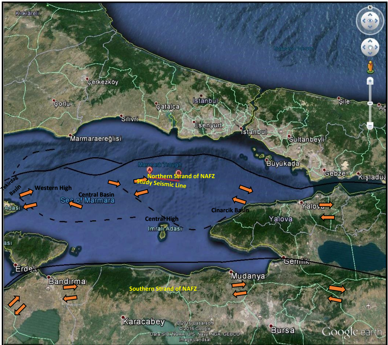
Figure 2 Regional fault map and tectonics of the North Anatolian Fault (NAF) System for the Marmara Sea. The seismic line used for this study, located along the central high, is and shown in red.
