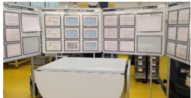
Figure 4: A Management Meeting Board on the Shopfloor with All Relevant Aggregated Shopfloor Data Displayed
