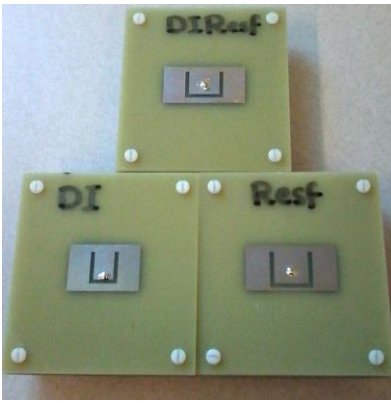
Fig. 3.6. Three prototypes of the probe-fed, U-slot microstrip patch antenna on \epsilon_r=4.4 (FR4) and h = 11.811 mm, finite, grounded dielectric substrate.
