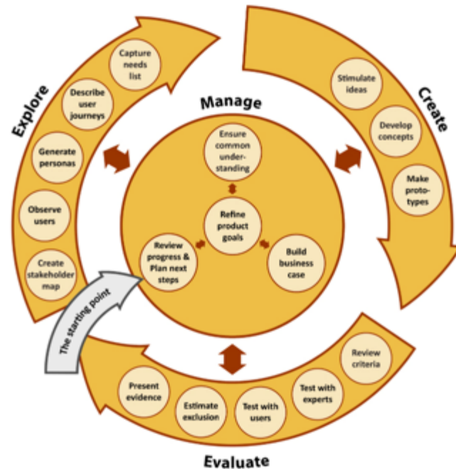
Figure 3-1. Phases and key activities of inclusive design. This diagram indicates key activities within the phases of inclusive design. Copyright 2015 by EDC. Reprinted with permission.
