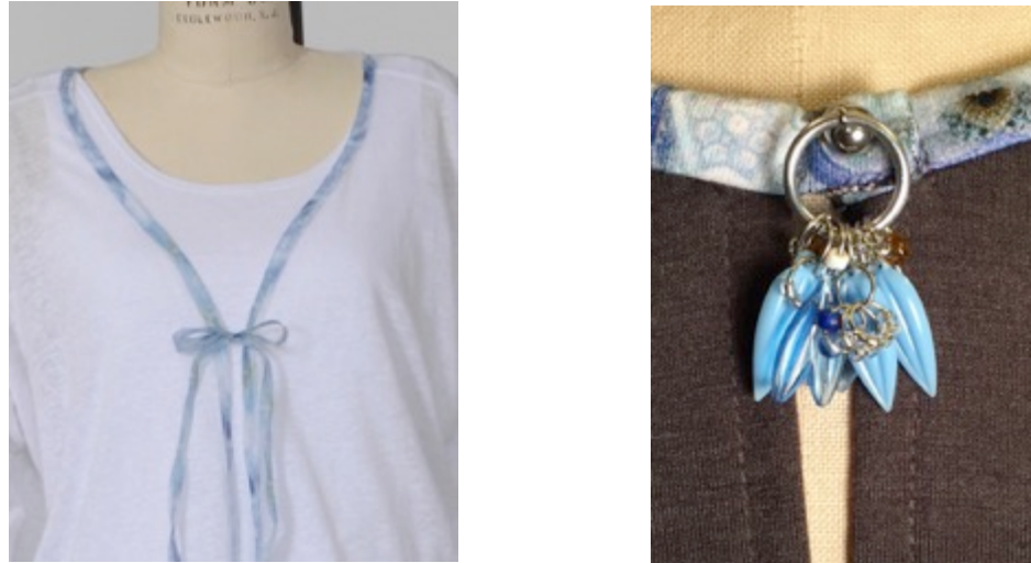
Figure 5-5. Silk organza print edge finish and tie (left) and cotton print edge finish with jewelry embellishment attached to the magnetic closure (right).
