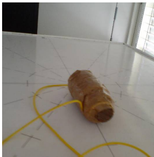
Fig. 5. Probe in horizontal longitudinal position
