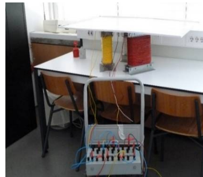
Fig. 2. Prototype built. The primary coils in delta geometric configuration
