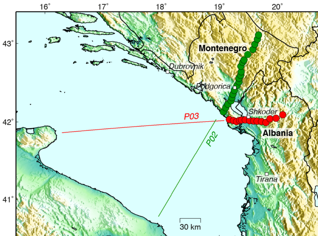
Figure 1: Topographic map of the ALPHA amphibious experiment. Lines P02 and P03 are the ship tracks, circles are the onshore seismic station locations.
