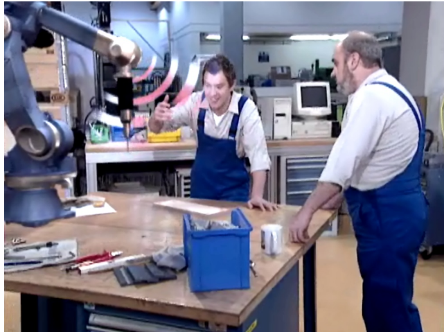
Figure 6.1: Illustration of industrial application of pHRI. The robot senses and reacts to the movements of the worker. © Fraunhofer IPA 2008
