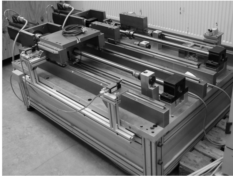
Figure 5.14: Mechanical setting of axis test rig.
