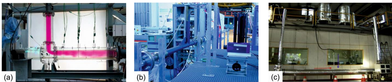
Fig. 7 Vattenfall [131] (a), MOTHER [4] (b) and EXTREME [17] (c) T-junction test facilities
