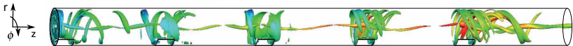
Figure 6.8: DES vortex structure in the MI5 swirl tube for Re = 10,000 , iso-surfaces of Q = 1 , color represents axial velocity
