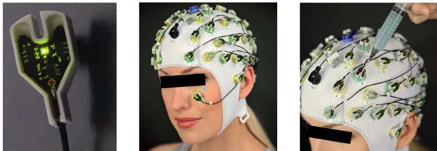
Figure 2.2.: ActiCAP measurement system for EEG recording by Brain Products GmbH (2009)
