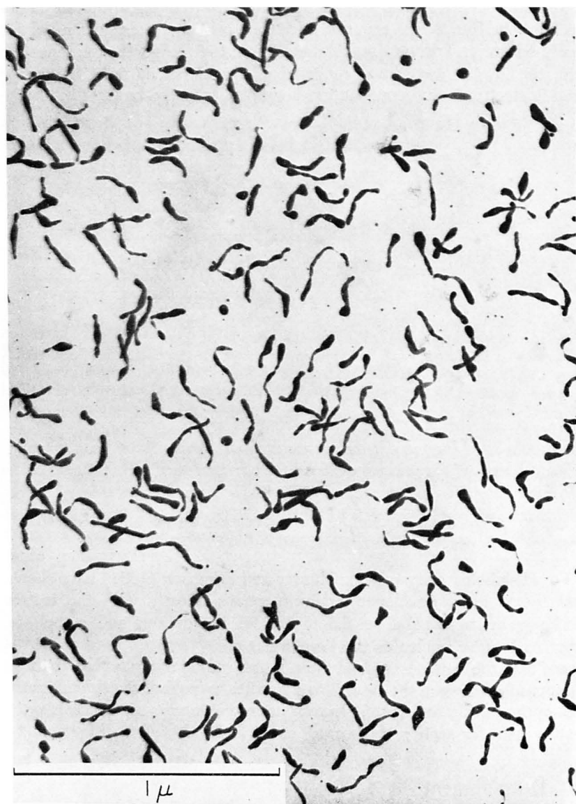
FIG. 3. Ilford L4 emulsion. Irradiation with 5.7 keV electrons in the AEG "SDL" electron microscope. Developed 1 minute in Microdol X. Magnification \times 53,000 .
