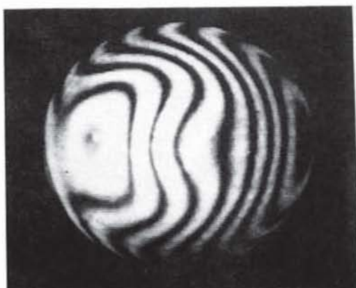
Fig. 9 A typical result of a testobject in reflexion with an off-axis CGH.
