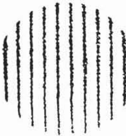
Fig. 3 Example of a complete compensation of spherical aberrations of a single plane-convex lens
