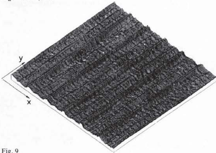
Fig. 9 Surface topography of a metal sheet surface with the mean roughness R_a = 1.59 \mu\text{m} , obtained with the fringe projecting microscope
