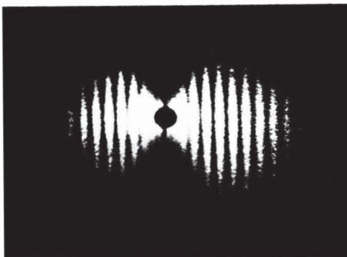
Fig. 7. Young's fringes obtained by recording the double exposure speckle pattern in the image plane with a displacement of 80 \mu\text{m} .
