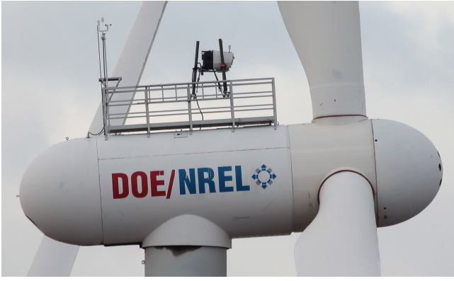
Fig. 1. The ZephIR DM lidar installed on the CART3 at the National Wind Technology Center. (Photo by Lee Jay Fingersh, NREL 32910)
