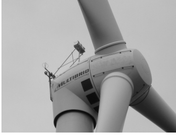
Figure 13: SWE nacelle-based pulsed LIDAR system installed on a 5 MW turbine [4].
