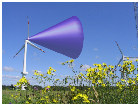
Figure 1: Sketch of a LiDAR system mounted on the nacelle of the MULTIBRID M5000
