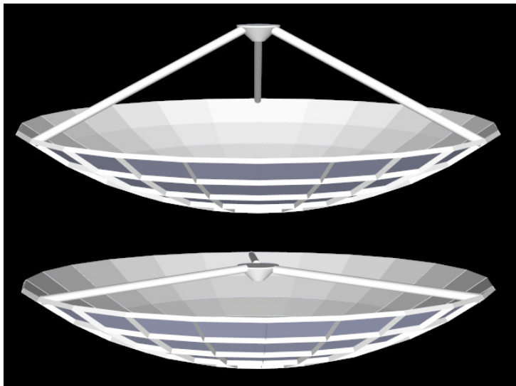
Figure 6-2: 1-meter parabolic dish in deployed and stowed configurations
