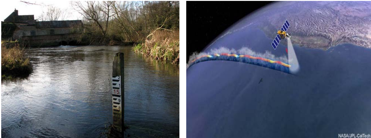
Figure 1.1 Example of traditional in-situ gauge measurement and satellite altimetry. We can see the limitation of in-situ gauge method, while the advantage of satellite remote sensing is its global water resources measurement and management.
