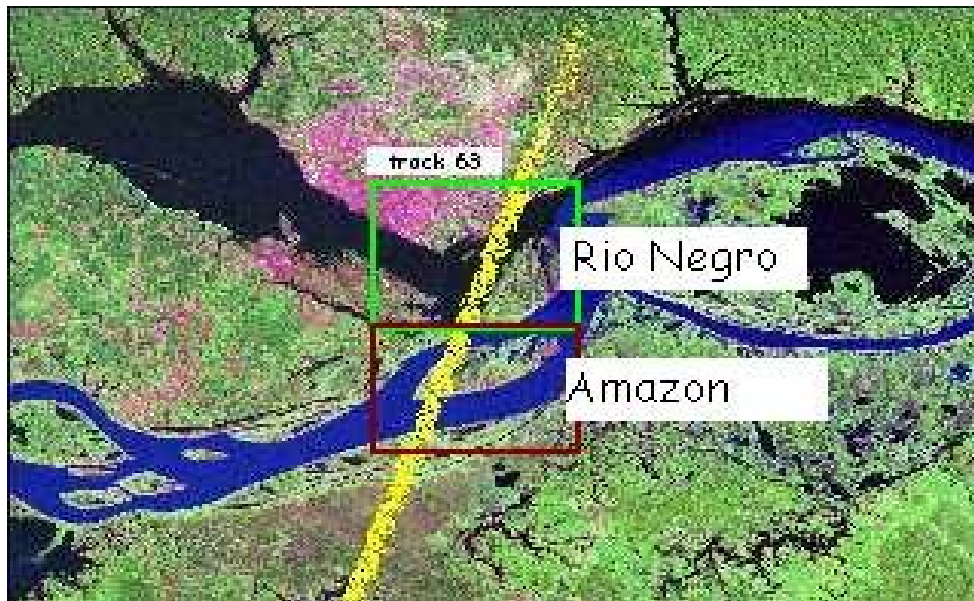
Figure 4.6 The Amazon River together with T/P track No 63. Since this section of river is only 5.7 km in width. So the number of 10 Hz footprint will be no more than 10, considering that inside the water body there are 2 island, corresponding waveforms (probably a half of them) are supposed to be noisy, which should be detected and removed automatically before waveforms retracking, aims at improving the data quality and better accuracy.
