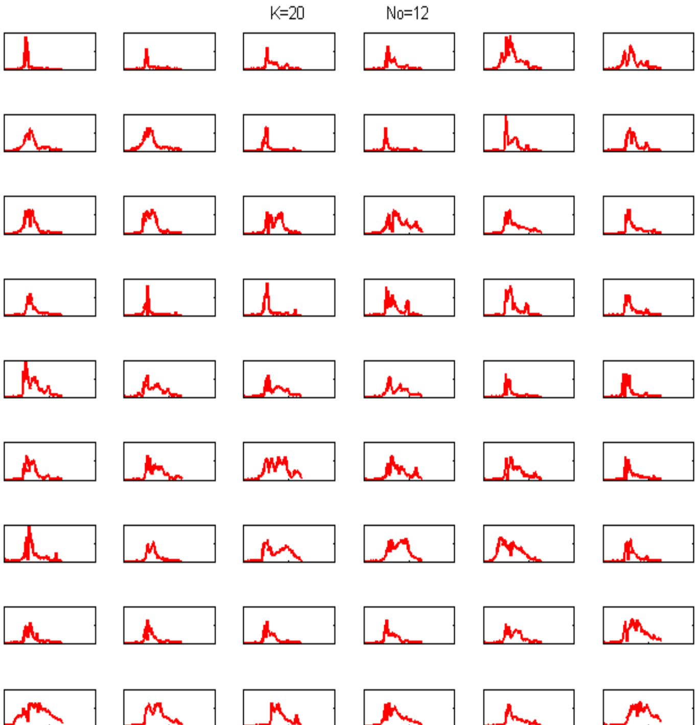
Figure 4.9 (a) K = 20 , N_0 = 12 In this group we set the threshold number of peaks to be 12, actually from the result it shows that 12 is a pretty big value, since still a lot of noisy waveforms exist after filtering, then we will try to use a smaller threshold value.
