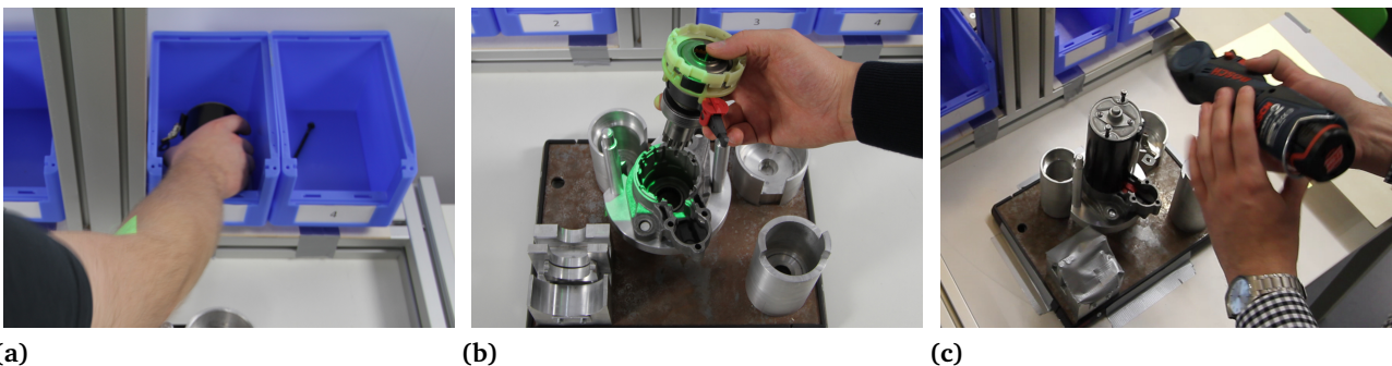
Figure 4.1: Indicators for steps: (a)Picking of a part from a box (b)Assembly of a part (c)Usage of a tool
