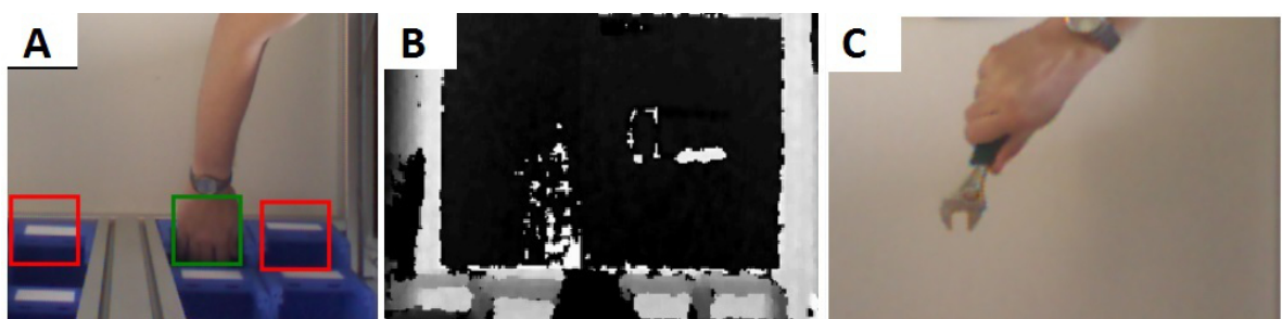
Figure 4.2: Triggers: A) Frame that monitors box depth data B) Depth image difference for assembly C) Image recognition for usage of tools
