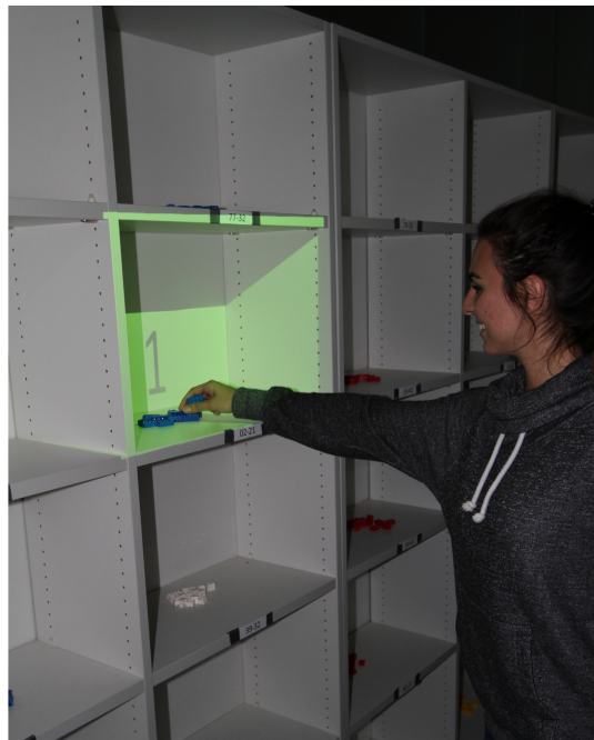
Figure 4.3.: A participant of our study, reaching into the highlighted box to pick up one item as indicated by the projection.
