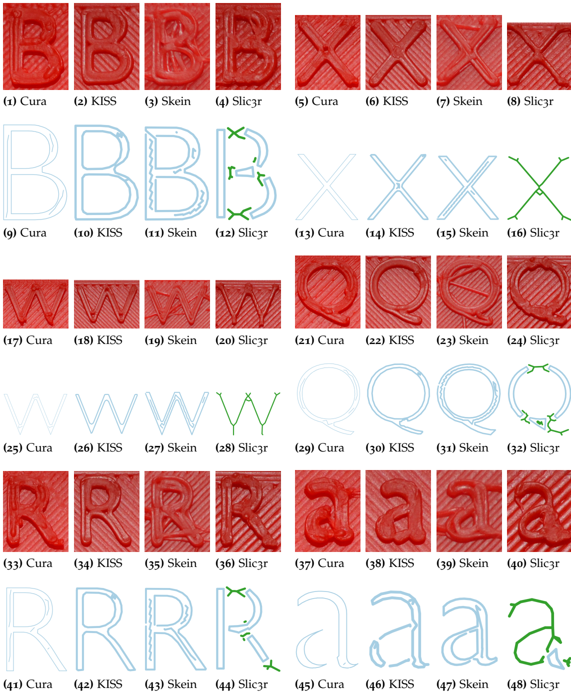
Figure 6.5: Selected letters of the Text Test with corresponding G-Codes. Used abbreviations: Cura: Cura, KISS: KISSlicer, Skein: Skeinforge, Slic3r: Slic3r
