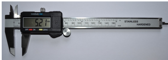
Figure 4.2: Caliper used for measuring the deviations
