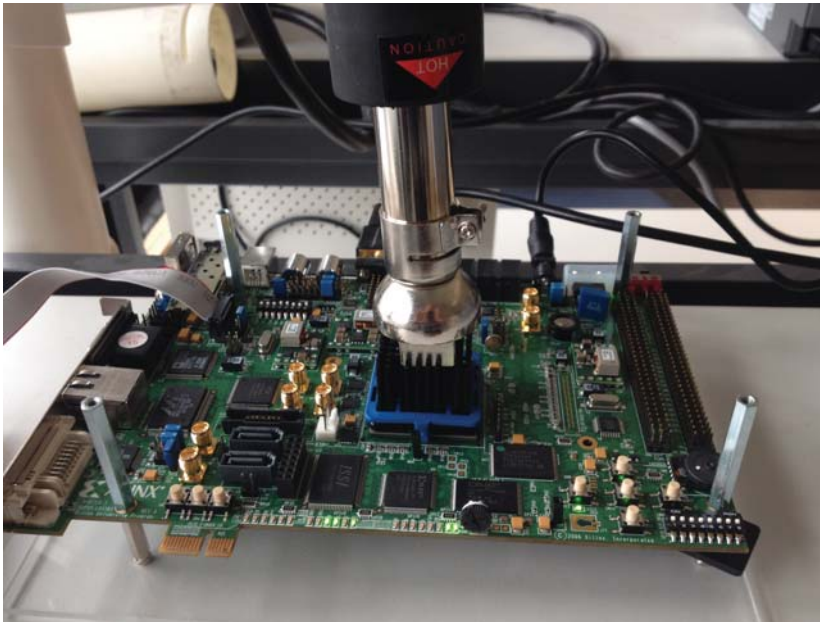
Figure 6.7: The experiment setup for external heating
