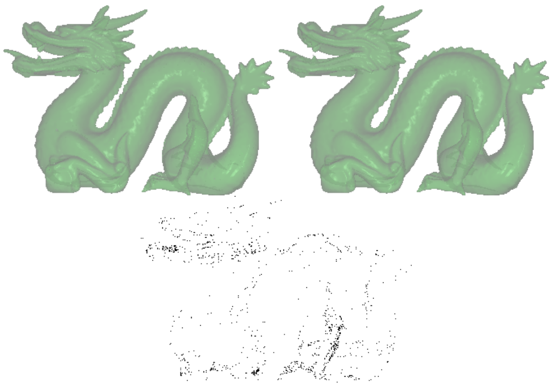
Figure 5.8.: Visual differences between images. Top left: image on display node. Top right: image on render node. Bottom: bad pixels which are different between the render node and the display node
