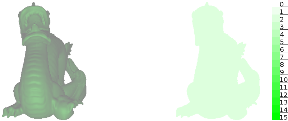
Figure 3.2.: Depth-limited rendering with 1 layer. Left: shaded; Right: number of fragments
