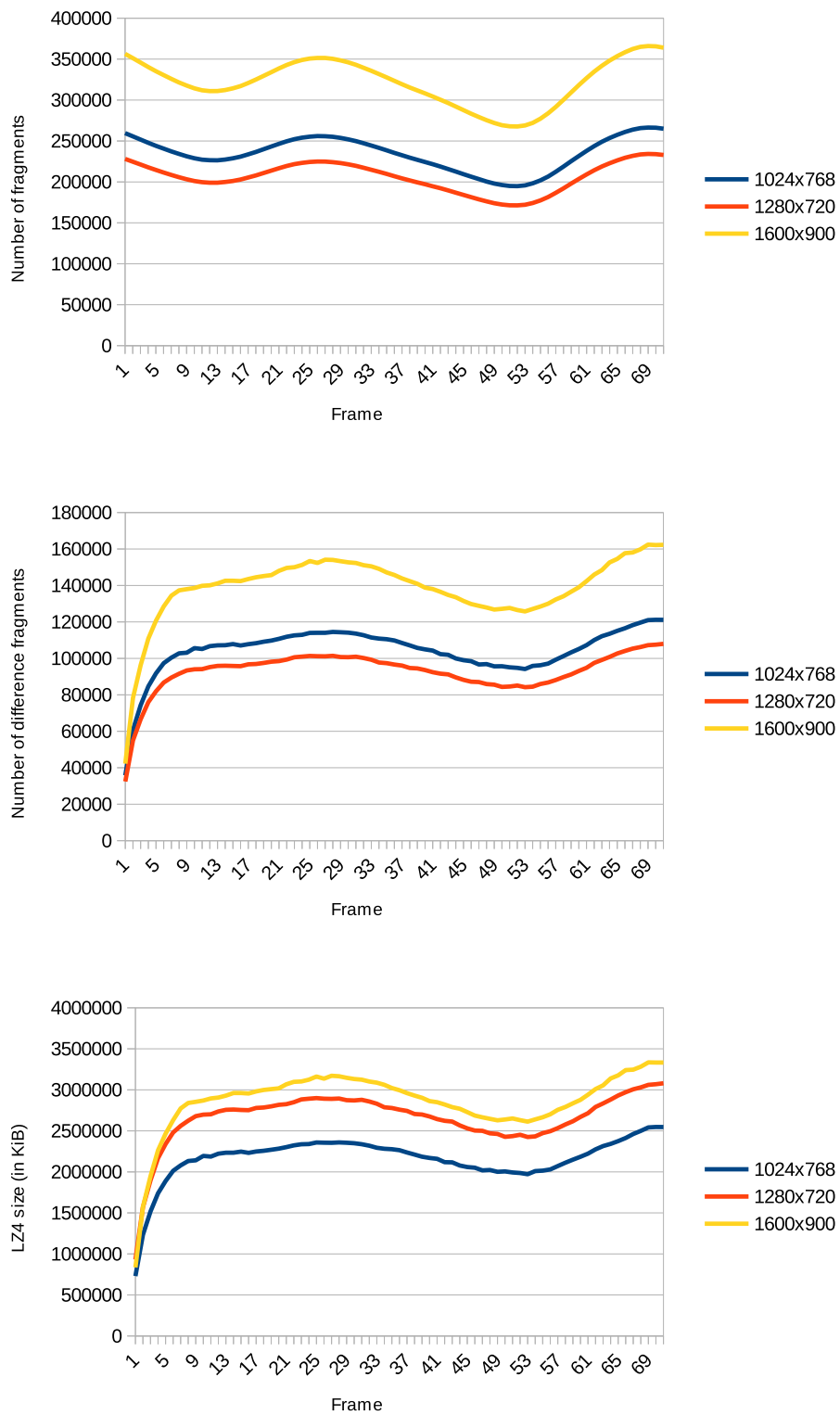
Figure A.4.: Network traffic using bilateral rendering for the bunny model with different resolutions
