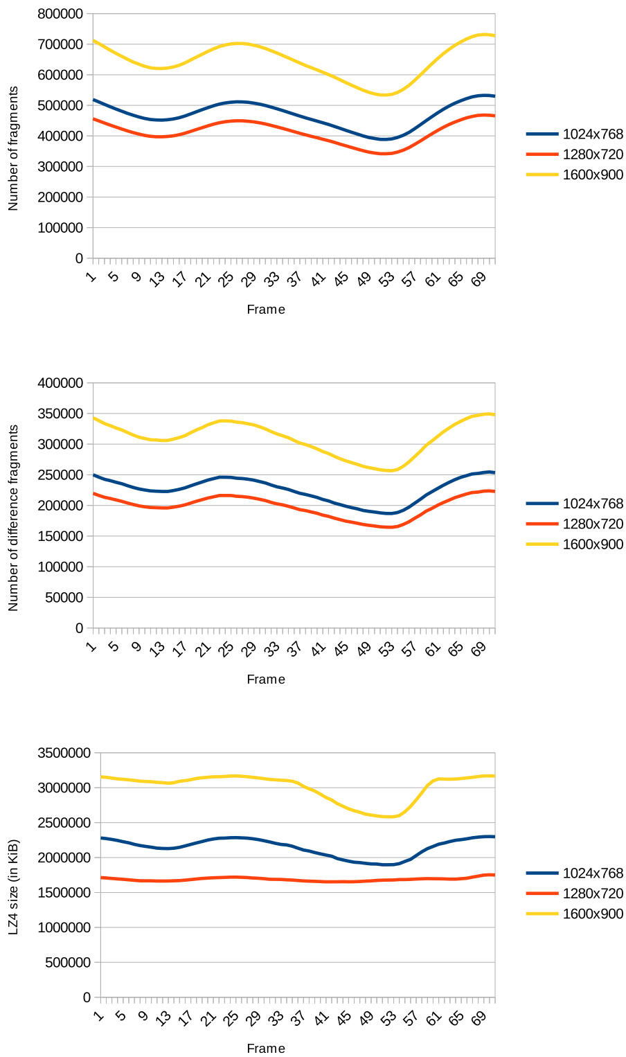
Figure A.3.: Network traffic using visual difference rendering for the bunny model with different resolutions
