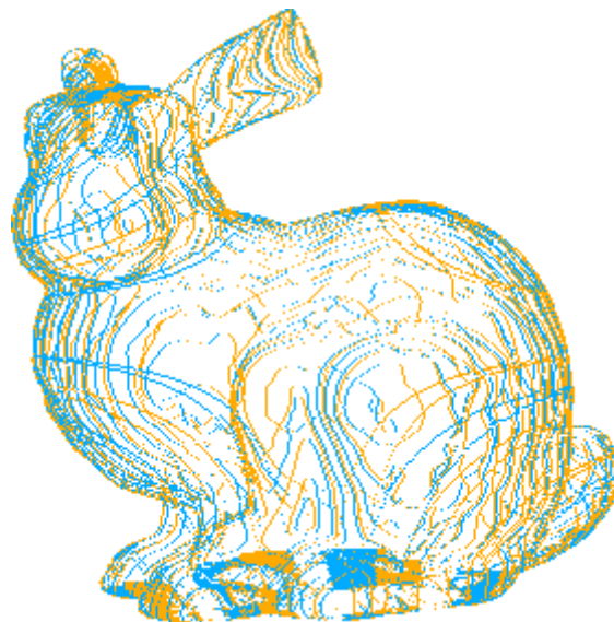
Figure 5.10.: Bilateral difference fragments, Orange fragments are to be removed, blue fragments are to be inserted.
