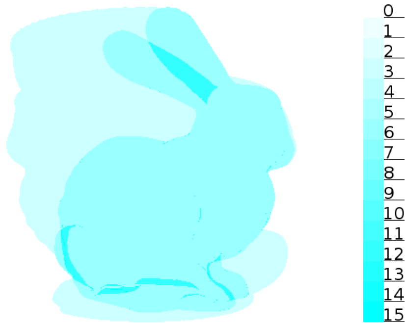
Figure 4.1.: Image showing the number of fragments for each pixel. The header will not point to 0 at positions where fragments were rendered before but to completely transparent fragments instead. Thus the number of fragments rendered on the display node is slightly higher than it is on the render node.
