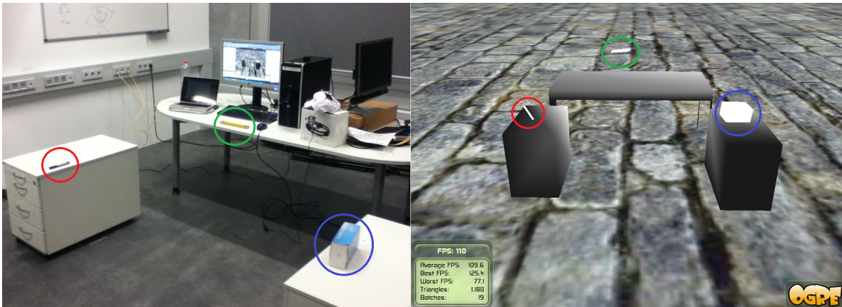
Figure 6.3.: Left side: The testing scenario in a lab environment. Right side: The corresponding 3D representation of the scenario. The colored circles show the correlation between a real-world object and its representation within the model.
