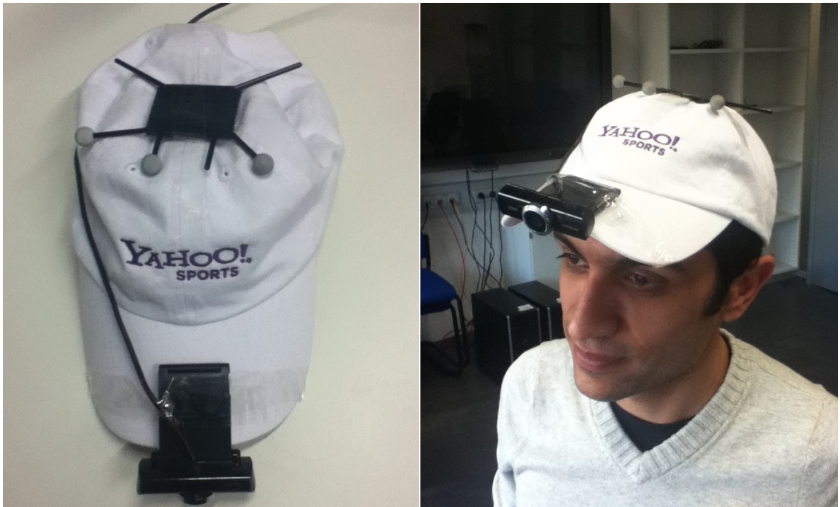
Figure 6.1.: The mobile Antonius prototype - a combination of a webcam, a marker and the user.
