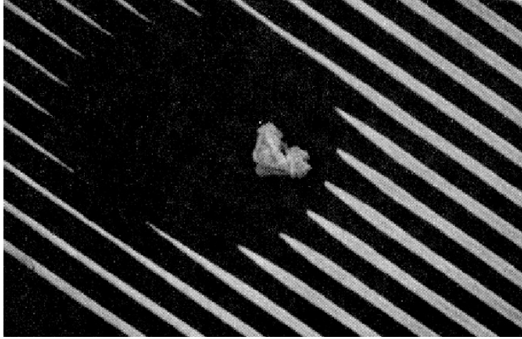
Figure 1.2: Example of a large break in a metal layer
