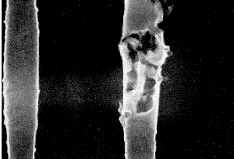
Figure 1.6: Example of a defect caused by metal corrosion
