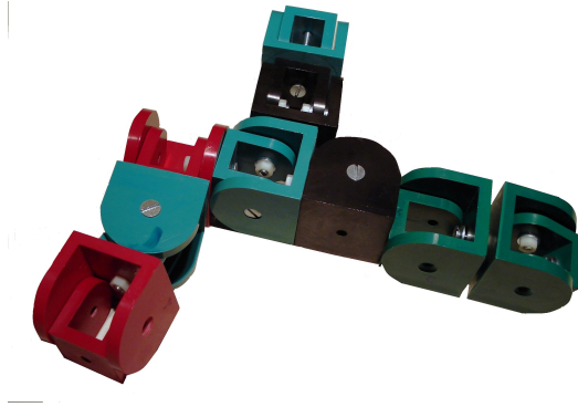
Figure 2.9: Modular Robot Assembly with n = 9 Modules and n - 1 = 8 Joints.
