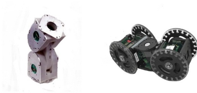
Figure 2.1: Two different Module Types both in Dyad configuration:(a)[iMobot, 2011],(b) [CKBot, 2009]
