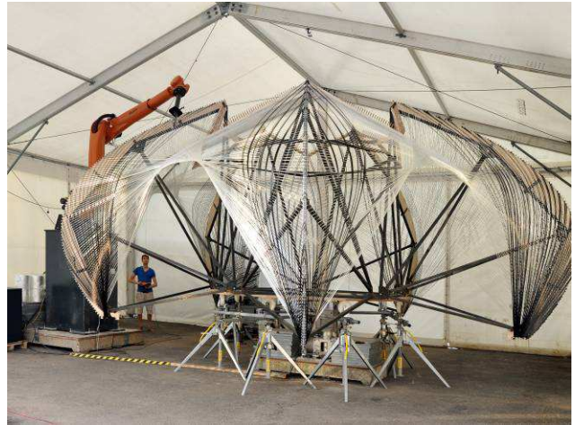
Fig. 5. Full scale test windings without resin
