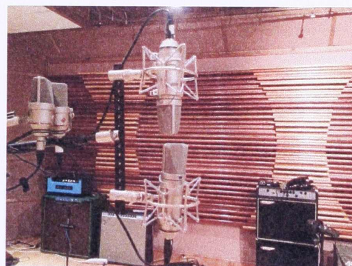
Figure 6: Blumlein bar for Blumlein stereo configuration. XY pair directly behind.
