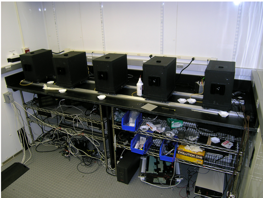
Figure 2.11: Photograph of DIH microscopes - five microscopes (black boxes) are shown on one half of an environmentally controlled room, in which temperature is 18 \pm 0.1 C.
