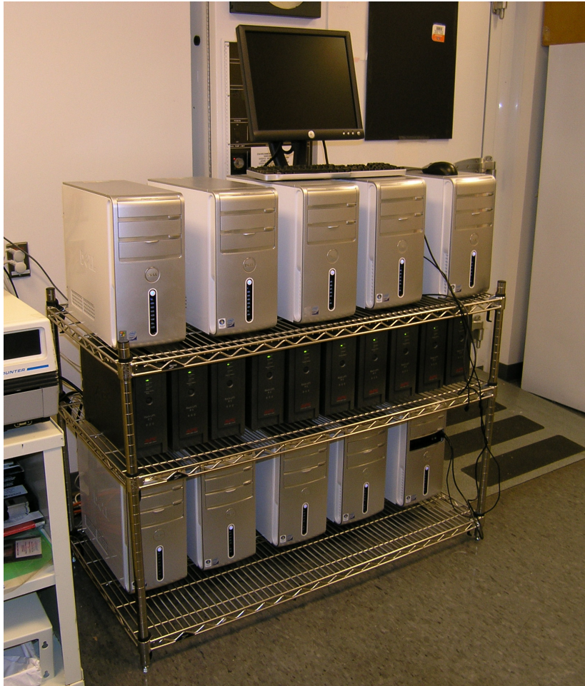
Figure 2.12: Array of DIHM computers - ten computers, one for each microscope, control the acquisitions, record voltages from the ADC and perform reconstructions and analysis. Each computer is powered by an uninterruptible power supply, and connects to its microscope through USB cables entering the environmental room through a small hole drilled in the wall.
