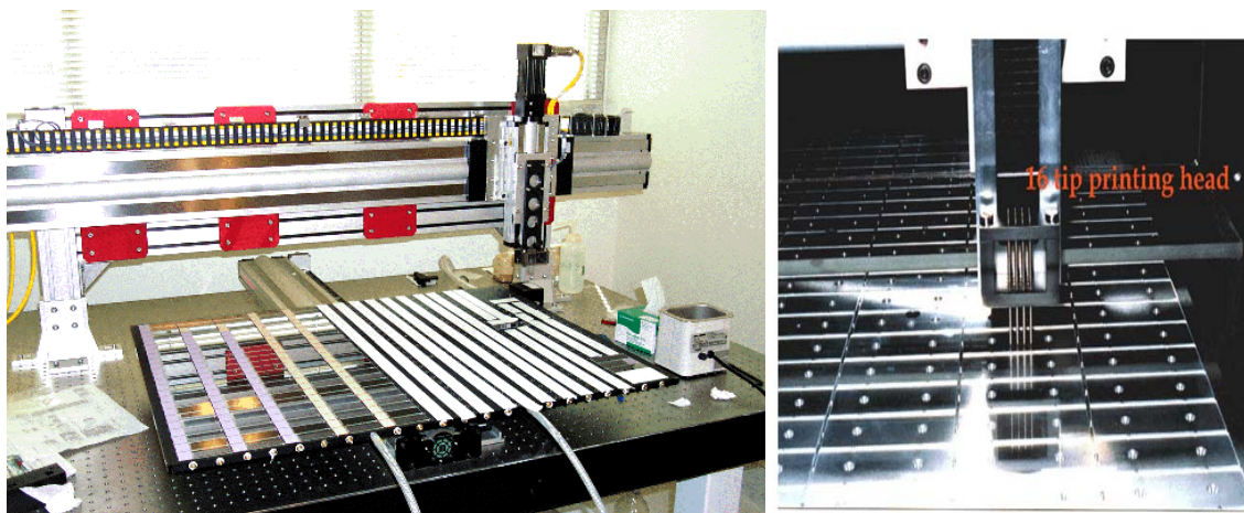
Fig. 1.2. Microarray printing robot from DeRisi microarrayer version II with 16 tip printing head. The microarray core from DeRisi Lab has recently assembled microarrayer version II. DeRisi's version II is capable of printing two batches per week, each batch containing 250 slides, with each slide containing a 40,000 spot array. (Adapted from DeRisi lab website http://derisilab.ucsf.edu/cshl/ )
