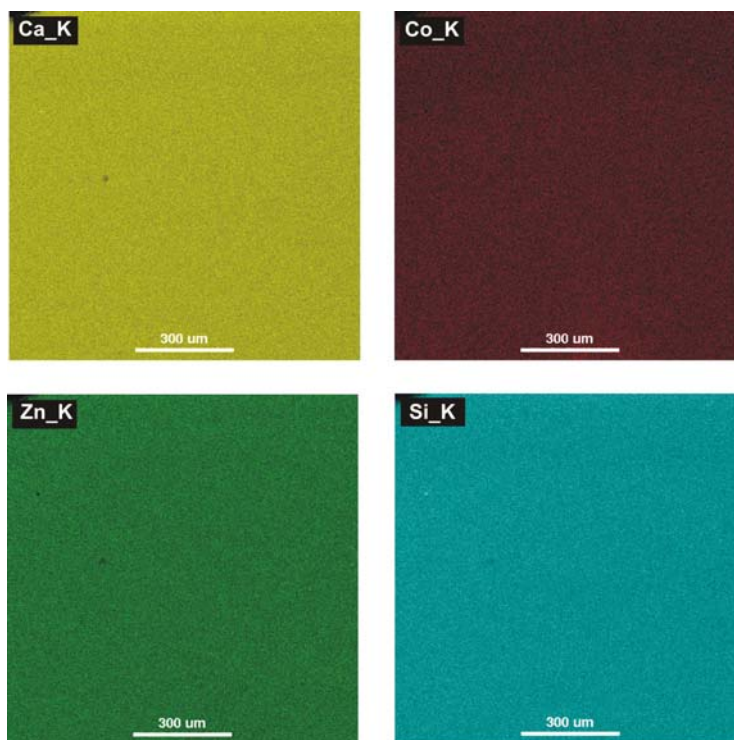
Fig.4.4.5 Density map of Ca, Co, Zn and Si elements in \text{Ca}_2\text{Co}_{0.9}\text{Zn}_{0.1}\text{Si}_2\text{O}_7 bulk crystal detected by EDS.
