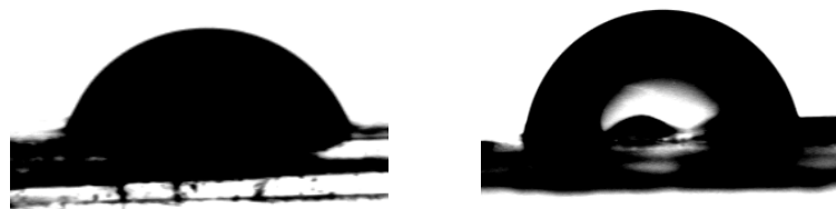
Figure 79. water droplets on the films; left, the contact angle of SH-mod-Sur-2 of the film, \theta = 72^\circ ; right, the contact angle of the film after thiol-stabilized-gold particles were immobilized onto the surface, \theta = 79^\circ .
