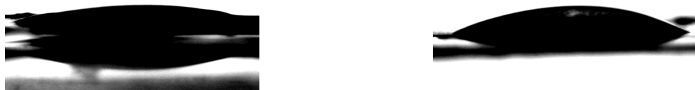
Figure 46. Water droplets on the films for one of the measurements: left, the contact angle of the H 2 SO 4 - treated-PPX film \theta = 12^\circ ; right, the contact angle of the H 2 SO 4 - treated-PPX film coated with a monolayer of PEI \theta = 22^\circ .
