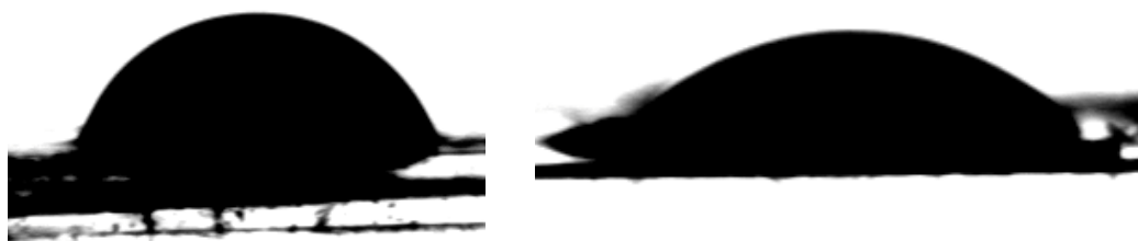
Figure 68. water droplets on the films; left, the contact angle of SH-mod-Sur-3 of the film, \theta = 72^\circ ; right, the contact angle of the film after DMAP-stabilized gold particles were immobilized onto the surface, \theta = 39^\circ .
