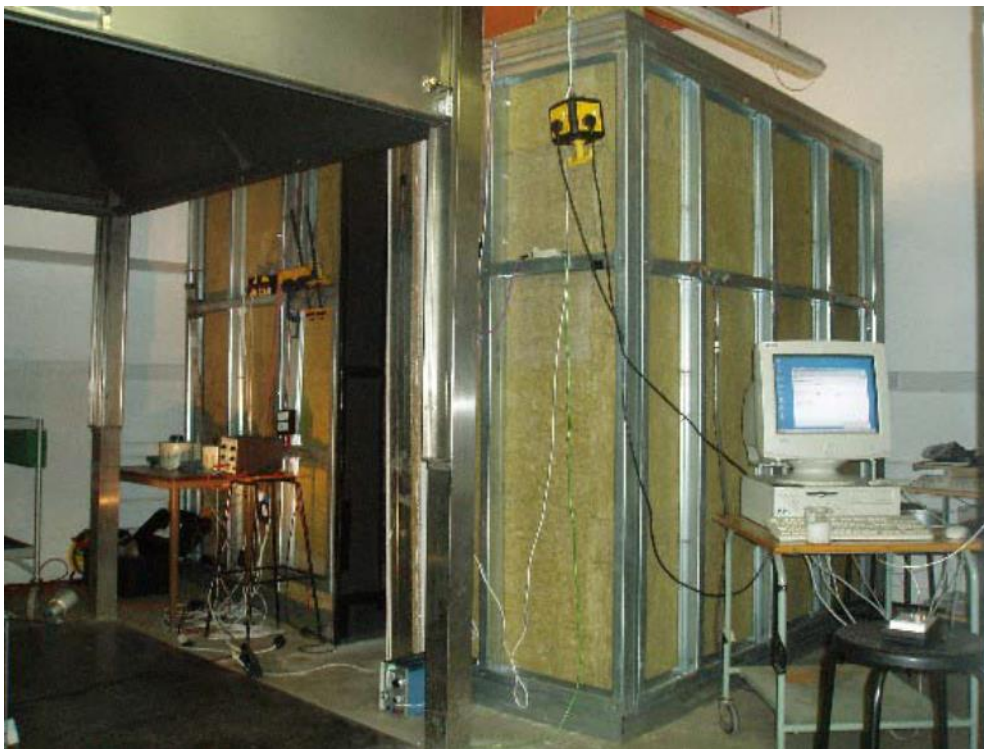
Fig. 17. Guarded Hot Box built by Amundarain.
