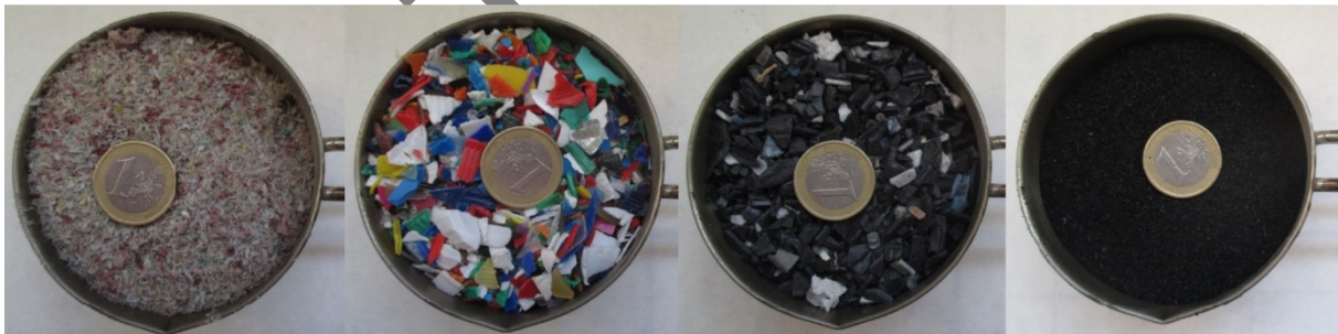
Figure 1. Selected polymeric waste: PE, PP, PS and ELT from left to right.
