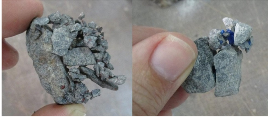
Figure 5. Coarse aggregates with PE and PP
