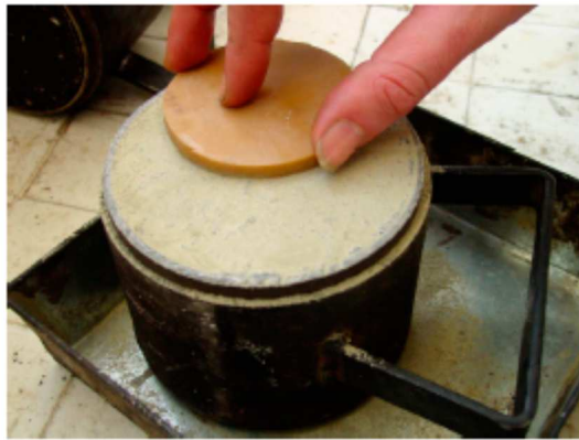
Fig. 2. Macro-texture measurement methodology.
