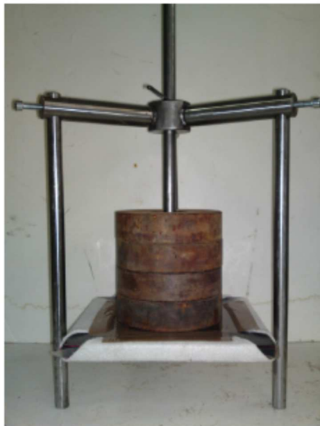
Fig. 10. Tack coat dosage control device.
