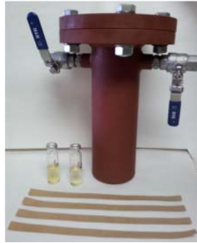
Fig. 7. Kraft paper strips and steel vessel.
