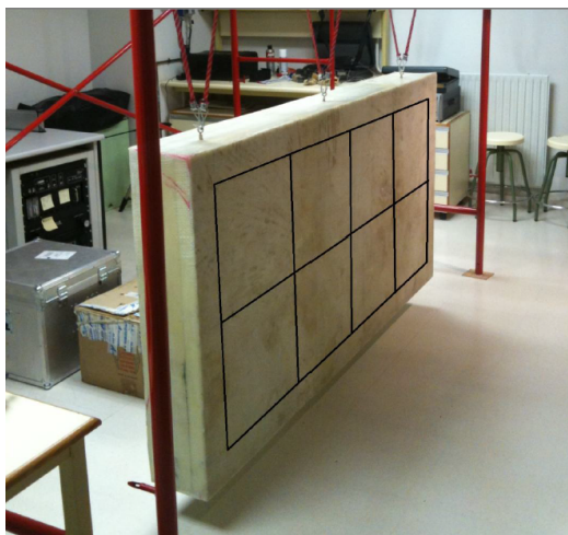
Figure 2: Boundary conditions and grid measurement of the sample MCS framework
