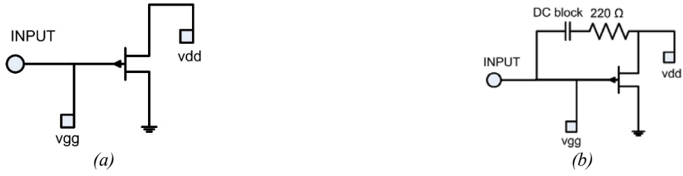
Fig. 7. (a) Schematic of a transistor, (a) common source, (b) common source with gate to drain feedback.
