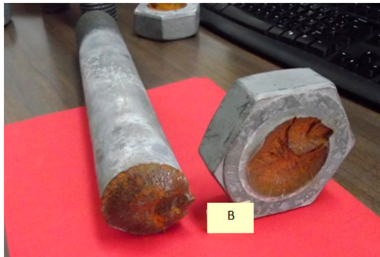
Figure 1. Bolt B at reception, showing the failure section.
