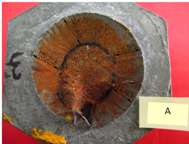
Figure 13. Approximate measurement of the external perimeter. Bolt A.
