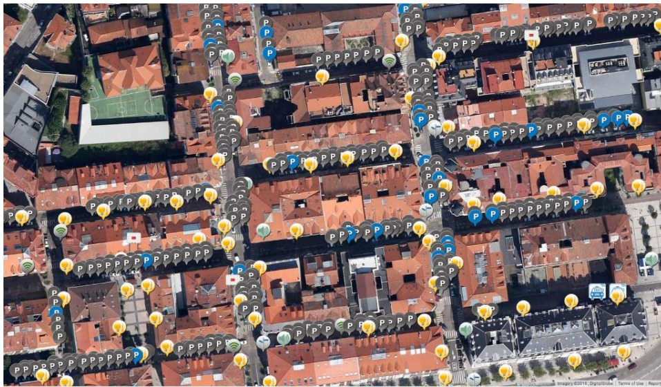
Figure 3. Detailed view of outdoor parking sensors deployment.
