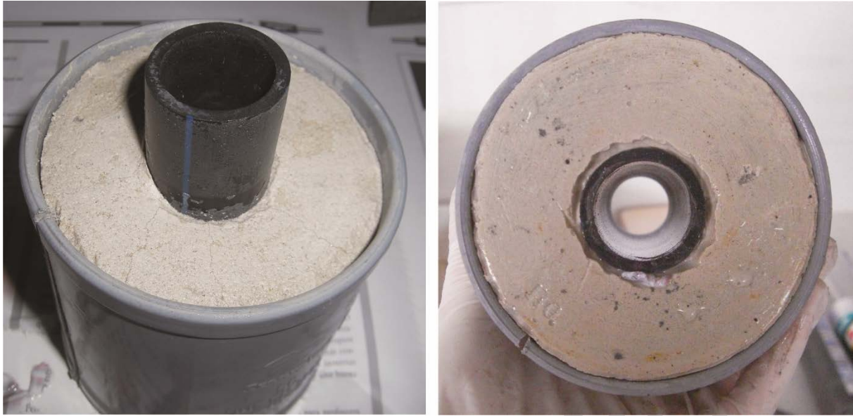
Fig. 12 - View of the grout-pipe specimen after 28 heating-cooling cycles.
